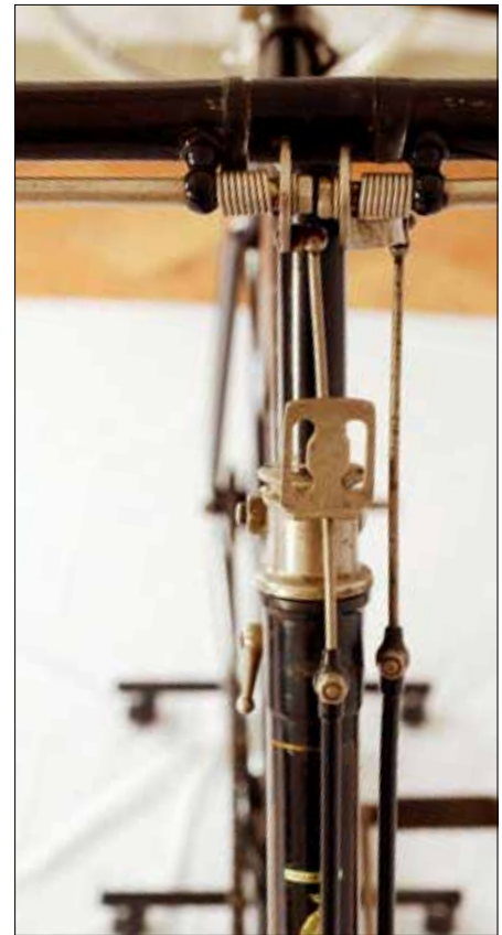
Figure 19. Handle bar detail of rigid mechanism use in Roller Brakes
