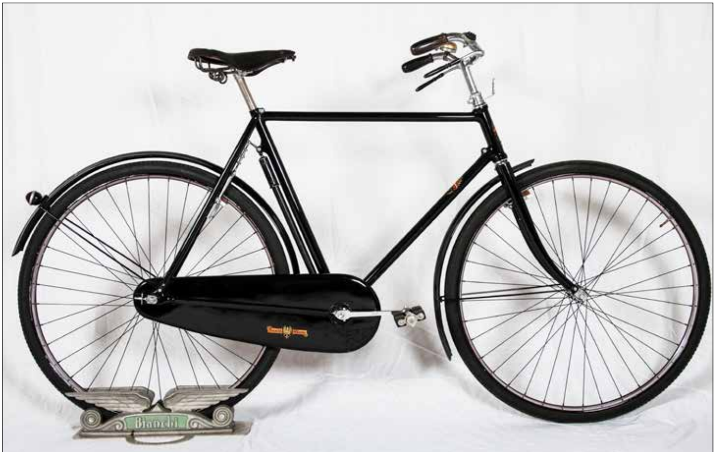
Figure 21. Bianchi R Super, 1928, with internal brake.
