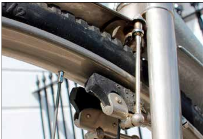
Figure 16. Front brake detail of Lea Francis, 1909.
