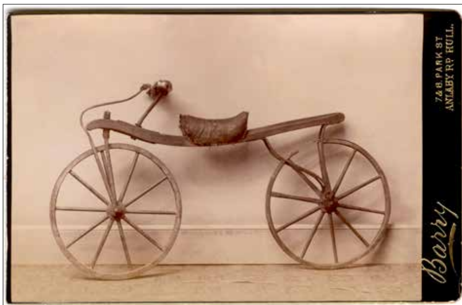
Figure 2. A FUN HOBBY Hobby Horse made in England. This style of vehicle was in general use between 1819 and 1823. The photo was taken much later and is from circa 1890. This type of cycle is commonly accepted as the first type of velocipede bicycle along with its older 'brother by another mother' the Draisienne as invented in Germany by Baron von Drais a few years earlier. There were no pedals or cranks. It had independent steering and similar sized wheels. It was a simple machine and worked broadly similar to a scooter. Cabinet Card albumen photograph. Photographer was Barry of Hull, England.
