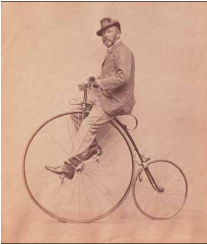
Figures 7 and 7a. A TRANSITIONAL TIME A Transitional High Wheel or Ordinary Bicycle made and mainly used within England and Europe. Photo circa 1873. Genre circa 1872 to 1875. A great example of an image showing the development away from the velocipede to the bicycle with the larger front and smaller rear wheels. The bicycle itself sports a mounting step on the rear fork, rear spoon brake, front tool bag, open head and Lallement style
