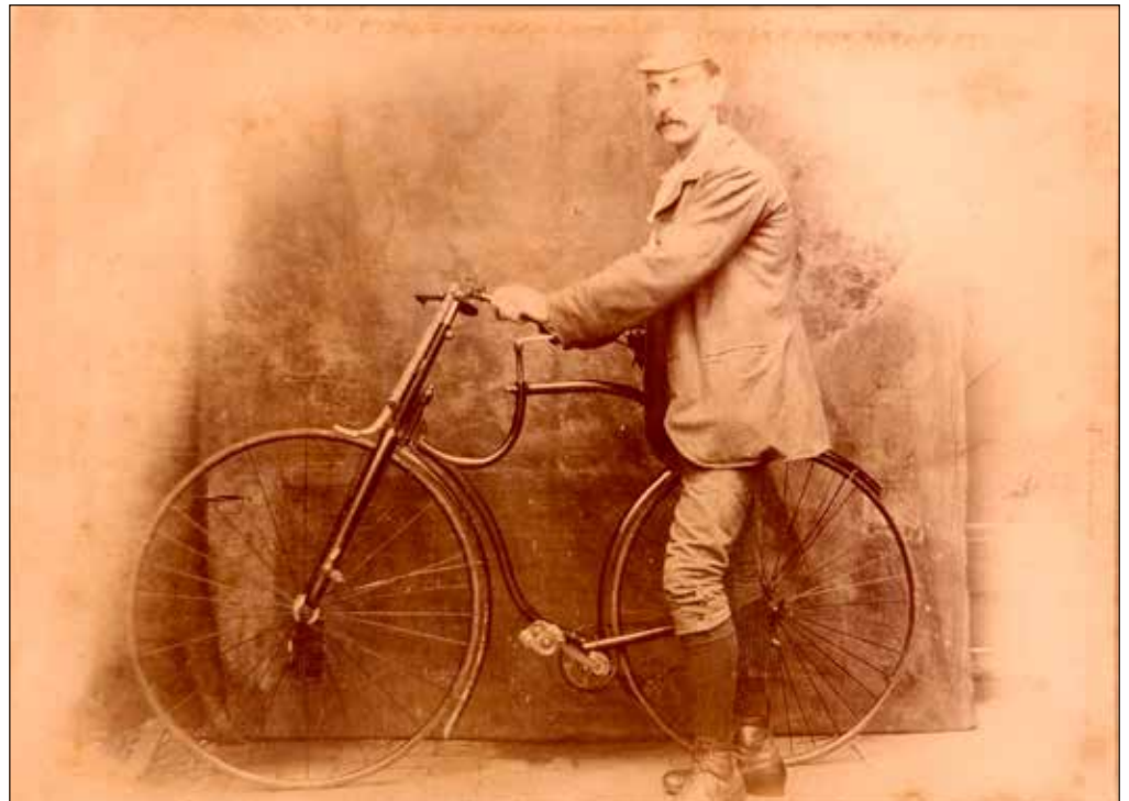
Figure 22. THE GREAT LEAP FORWARD The Rover safety. A hearty welcome to John Kemp Starley's Rover. Photo circa 1887. On the market circa 1885-1890. Exported worldwide. This rear wheel drive cycle with two similar sized wheels on a 'diamond frame' dramatically enhanced the stability and ease of riding. It "set the pattern to the world". The factory, "Starley & Sutton" created the name Rover, which was first used on tricycles in 1883. This was not the first pattern Rover safety bicycle, but the 3 rd generation. It had developed very rapidly to the diamond frame. In contemporary script on the reverse it identifies the rider as: Joseph Burton Stubbs, High St, Congleton. The Capitol Cycle Co. in Washington DC was their American distributors. No photographer identified. England
