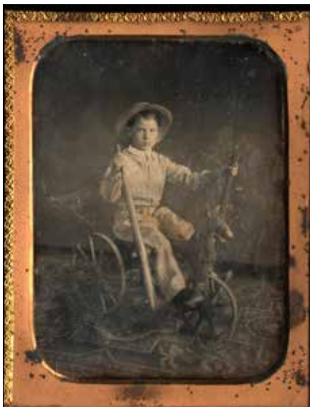
Figure 3. A PROPELLER BY ANY OTHER NAME IS A VELOCIPEDE In contemporary times, this vehicle was called a Propeller or Velocipede. The photo is dated 1850. This genre vehicle was in use from the late 1830s to the early 1860s. This manumotive tricycle was produced in the USA, and similar machines were found in Canada and England. The vehicle is driven by levers activating the rear axle causing the rear wheels to rotate. The velocipede was steered by the feet by putting pressure on pegs at the front wheel. The youth is identified as Frank Bakewell James of Cincinnati, Ohio. He eventually became a colonel in the Civil War. At this time, it is the earliest known dated photograph of a manumotive/pedomotive velocipede/cycle with provenance confirming the date. The photograph itself is a 1/2 plate Daguerreotype housed in a folding hinged case. Unknown American photographer.
