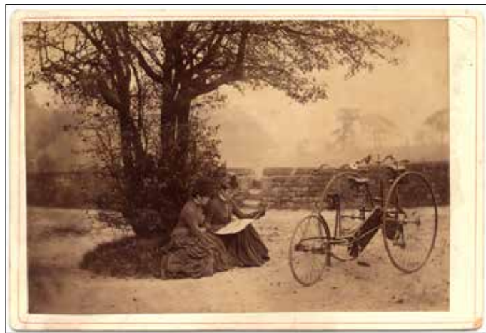
Figure 10. WHICH ROAD WOULD YOU CARE TO TAKE? Quadrant Tandem Tricycle, England. Sold in England, Europe and North America. Photo taken ca 1886. Genre ca 1884–1889. A box HTS lamp, Luggage carrier straps and bell adorn the tricycle. Quadrant tricycles were very popular and had a smooth ride in large part because of the front channeled wheel system. The ladies seem relaxed and enjoying their read of the map. Perfect hats to spotlight those of the era. Where to go next? A well composed image of a perfectly chosen mid-1880’s ladies cycling scene. No photographer’s identification. Albumen cabinet card.
