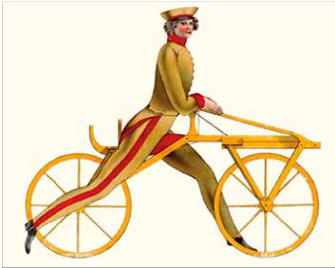
Figure 2. A Draisine from 1817 invented in Karlsruhe, Germany. The Rider moves forward rapidly on land using a skating motion with his feet on the ground.
