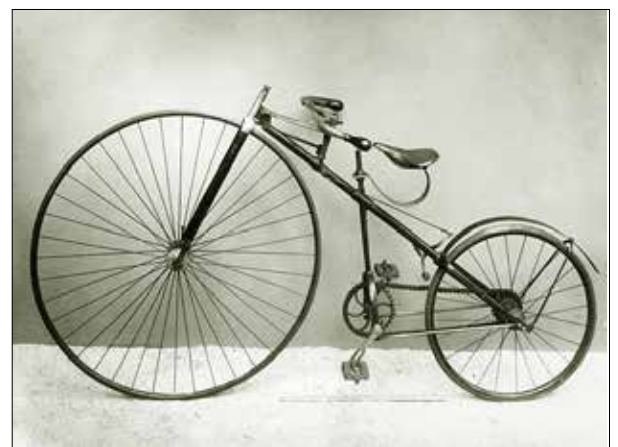
Figure 7. "La Bicyclette" designed by Harry J. Lawson when he worked for the Rudge Cycle Company in Coventry, England, in 1879. These bicycles were sold in France and other countries in Europe, and their name became established in France as the name for all Safety Bicycles thereafter.
