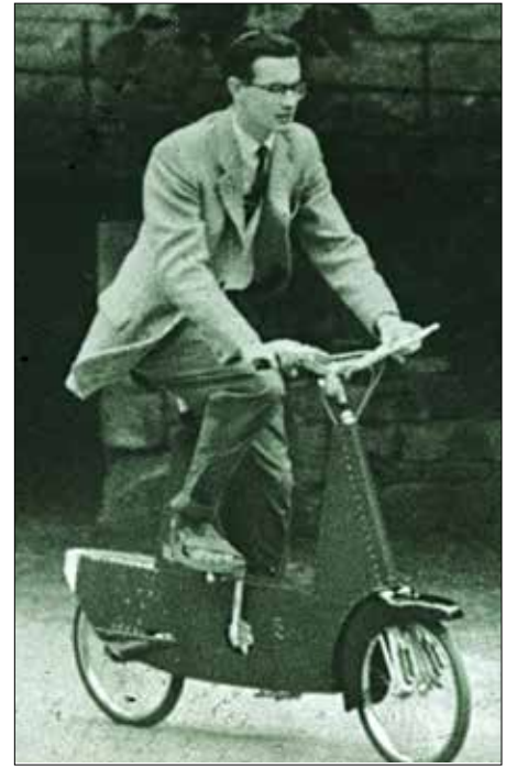
Figure 3. The first rideable prototype of the Moulton bicycle- monocoque construction, the 'noisy bicycle'. Courtesy of the Moulton Bicycle Company.
