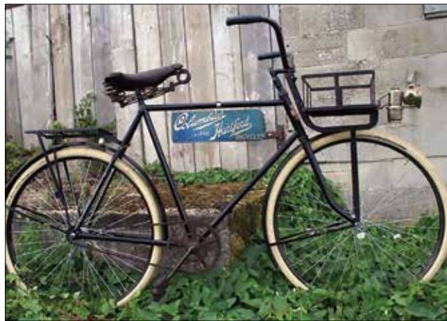
Figure 7. 1912 Pope Daily Service Bicycle manufactured by Columbia. Note the heavy-duty racks that came as standard equipment. Photographer and owner Colin Kirsch, www.oldbike.eu
