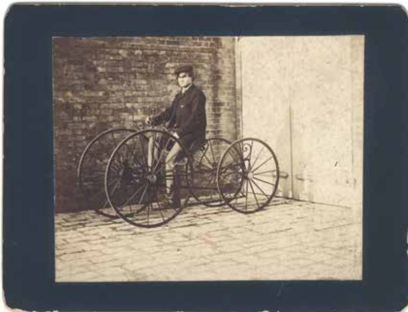
Figure 3. A SAWYER QUADRICYCLE - GENTLEMEN, I AM READY Henry Hill Hodgson on a Sawyer Quadricycle (see similar photo in King of the Road by Andrew Ritchie p. 42). Hodgson was a bookseller and auctioneer, having his sales room at 115 Chancery Lane in London. He first acquired his Sawyer Quadricycle in 1856, which he rode consistently for extended distances. Selected because it illustrates an early front-drive, rear-steering Quadricycle. Identified as Henry Hill Hodgson on the reverse. These early historic vehicles originated in England. Much more information about Hodgson is available from the Museum of the History of Science in Oxford. Circa 1860. No photographer's identification. Size of mount is 4-1/8" x 3-1/8". Albumen photograph mounted on board.
