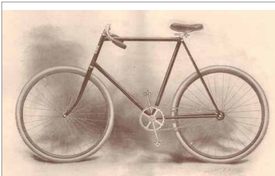
Figure 12a. Crawford Men's Bicycle, 1897. Note that the drive train is on the cycle's left side. (Crawford Bicycle Catalog, 1897).
