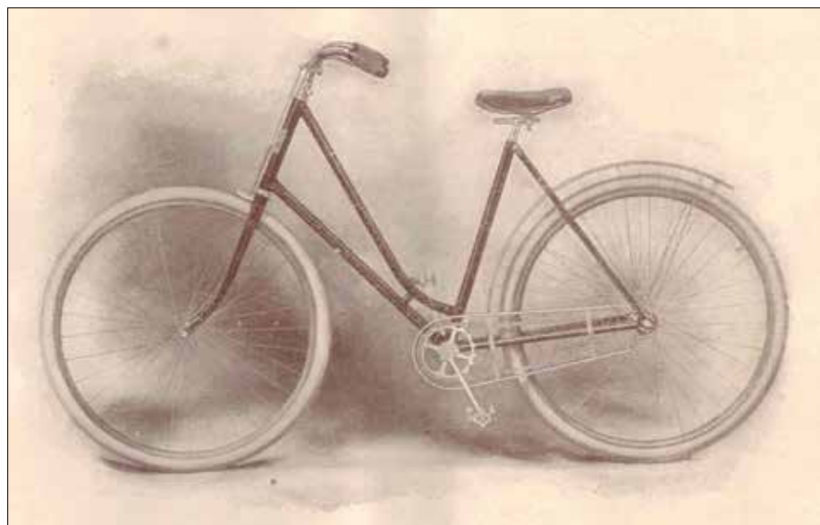
Figure 12b. Crawford Ladies Bicycle, 1897. Note that the drive train is on the cycle's left side. (Crawford Bicycle Catalog, 1897).
