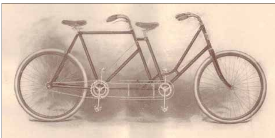
Figure 12c. Crawford Tandem Bicycle, 1897. Note that the drive train is on the right side of the tandem. (Crawford Bicycle Catalog, 1897).
