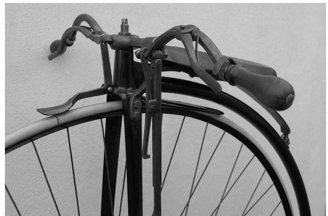
Fig. 5.1. Handlebar hand-cranking detail of Barták high-wheeler.
