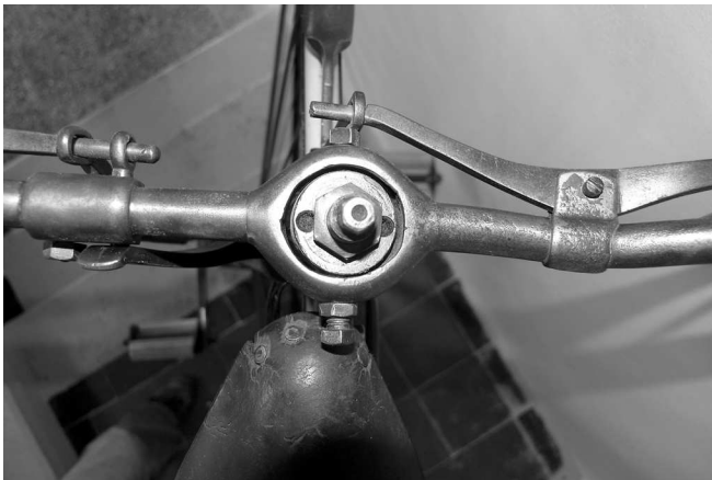
Upper left: Fig. 5.2. Handlebar fixing pin detail.
