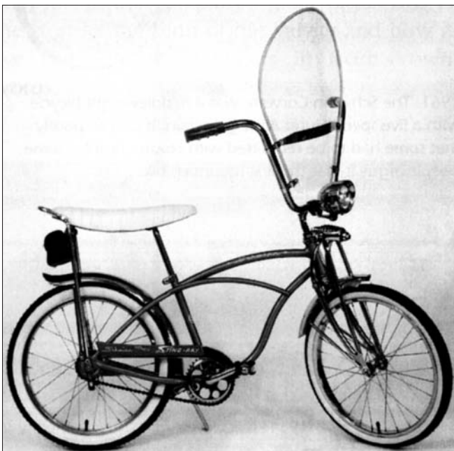
Fig. 1502. Schwinn Sting-Ray, showing the banana saddle, sissy bar, and longhorn handlebars. This de Luxe model is also equipped with a 2-speed coaster brake hub, lights, and a windshield.
