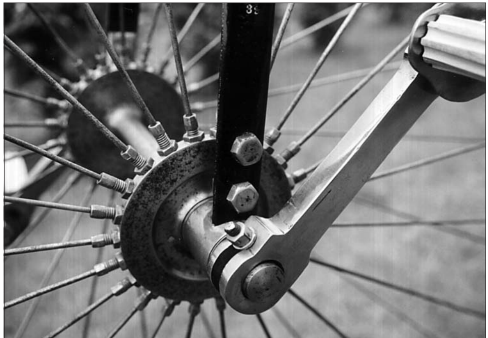
Fig. 0201. The hub with roller and crank of the Kohout No. 39.
