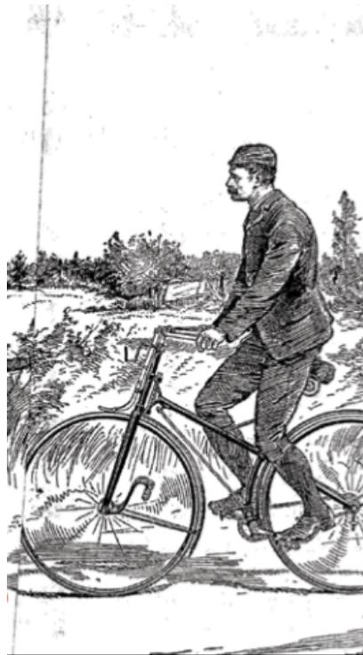
Figure 1. An 1887 Rudge Cross Frame Safety Bicycle with direct steering. This picture is from an ad for this bicycle in *The Bicycling World*, 30 September 1887, p. 403.
